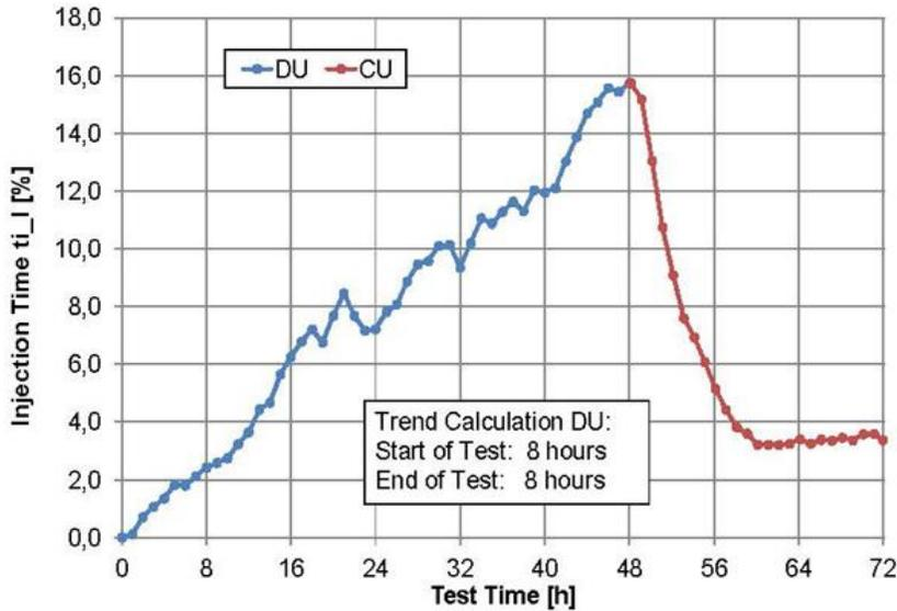
Looking at the Dirty-Up (DU) portion of the curve (in blue), we see immediate deposit formation as soon as the test begins. By the time the engine has run only 8 hours, injectors are already remaining open 2.2 percentage points (pct pts) longer in order to deliver the same quantity of fuel to cylinders. At 16 hours, this has increased to over 6 pct pts longer, culminating in an almost 16 pct pt increase in injection time by the time the DU phase concludes at the 48 hour mark.
