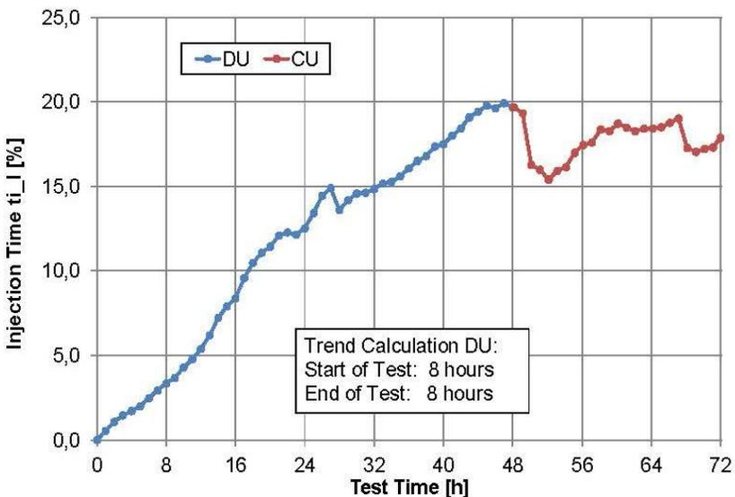
Looking at the Dirty-Up (DU) portion of the curve (in blue), we again see immediate deposit formation as soon as the test begins. By the time the engine has run only 8 hours, injectors are already remaining open 3 percentage points (pct pts) longer in order to deliver the same quantity of fuel to cylinders. At 16 hours, this has increased to over 8 pct pts, culminating in a 20 pct pt increase in injection time by the time the DU phase concludes at the 48 hour mark.
