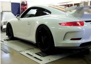
Results were: Baseline, without additive: 410.7 hp. With friction modifier: 426.3 hp. Therefore, a gain of 3.8%.
