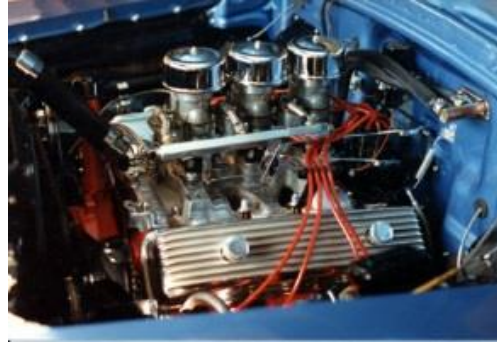
The motor in our Olds, a 324”mill with 3x2 Weiand aluminum intake manifold and progressive linkage, protected by No-Rosion (or CWT-37) for 35+ years.
