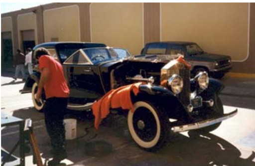
Converting the cooling system of Mr. Nethercutt’s 1930 Rolls Royce Phantom II Brewster Town Car to a mixture of No-Rosion and reverse osmosis (RO) water.
