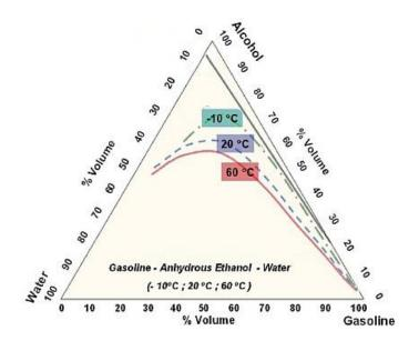
Detailed investigative laboratory analysis has been conducted to study the relationship between gasoline, ethanol, and water. The results are best demonstrated by what is referred to as a **Ternary Phase Diagram**, as pictured at left.
