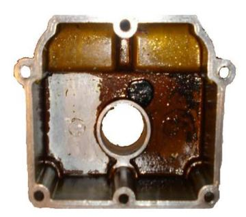
At left is an image of a carburetor float bowl from a 1967 Jaguar XKE. The tank of this car was filled with gasoline that was later determined to be a high RVP winter blend. It was parked in a climate-controlled garage for 20 months. The gasoline evaporated from the carburetor, leaving behind heavy, sticky <u>gum</u>s. The gums were bad enough to prevent the carburetors from functioning, and the car would not start or run.
