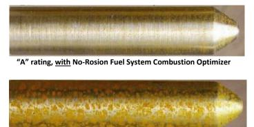
"E" rating, without No-Rosion Fuel System Combustion Optimizer
